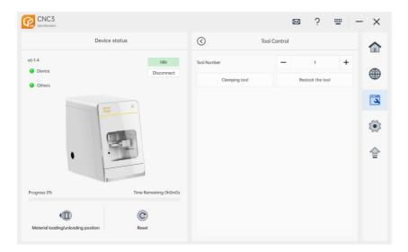
Clamp Tool: Select any tool number, then click "Clamp Tool". The machine will grip the tool corresponding to the selected tool number.
