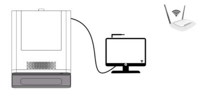
Connect to the computer with UPCNC installed via the local network (converter).
