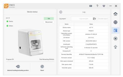
Log Export: Click on Log Export, select the export path, and then click Export All to export all log information of the current machining machine, including the lower machine log, device information, operating environment, Link information, current NC file, machining machine parameters, and upper machine log.
