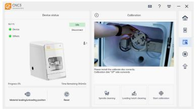
Spindle Cleaning: Clicking on "Spindle Cleaning" moves the current machine to a specified position and opens the chuck.
