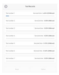
Reset: After selecting any tool, clicking on "Reset" will reset the current usage record.
