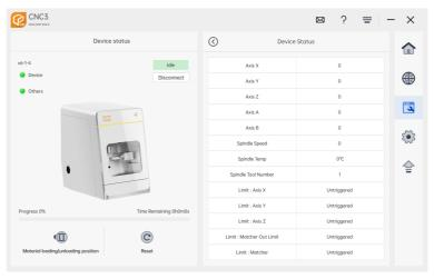
Device Status: Displays the current coordinates of each axis on the machining machine and whether limit switches are triggered.
