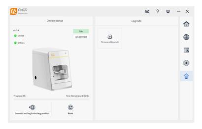
Restart Device Upgrade: As shown in Figure 4.1, after entering the firmware upgrade page, select the corresponding upgrade package and click "Restart Device Upgrade." This will erase the current firmware of the machine, switch it to BOOT mode, and require reconnection to BOOT mode.
