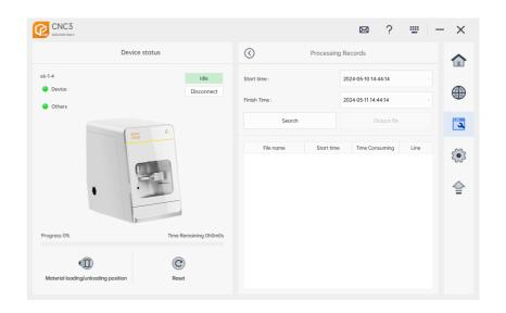
Start Time and End Time: Displays the start and end times of historical NC processing. Clicking on it opens a dropdown menu where you can select the historical processing time and start time.
